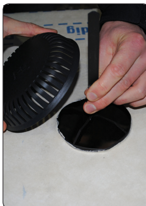
Mount the grill, whilst holding onto the strip
